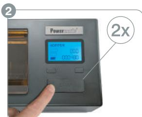
Wait until HOPPER appears. Press START again and wait for the spoon to come out. When the spoon is fully out, quickly press START for the second time.
